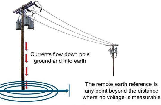
Voltage Gradients Appear Across Earth's Surface Near Point of Current Flow
